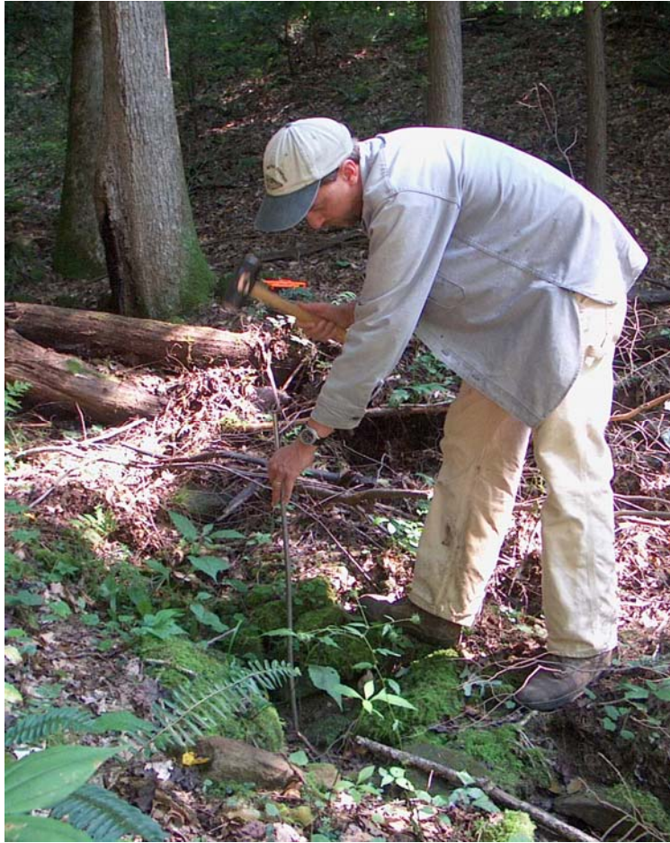
Figure 3-51 Using sounding rod and hand sledge hammer to estimate depth to bedrock and the groundwater table.
