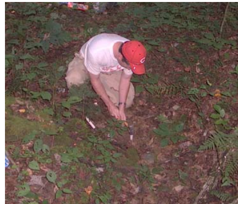
Figure 3-55 Tapping core vertically into streambed.
