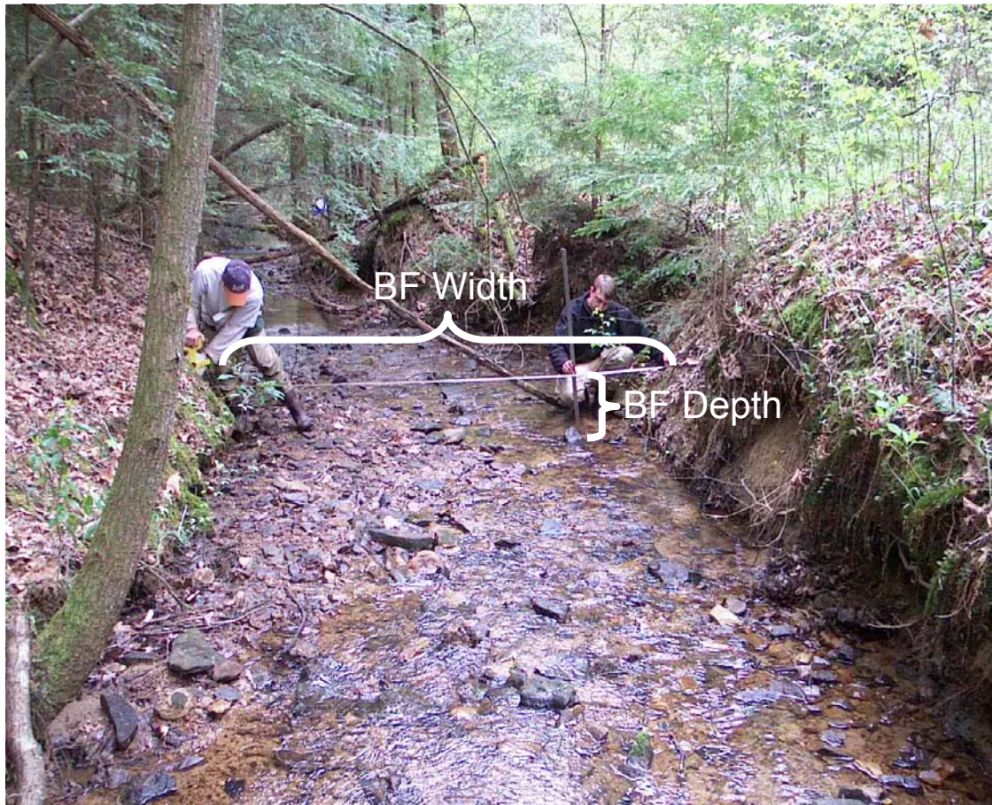
Figure 3-37 Photograph shows measurement of bankfull (BF) width and bankfull depth.
