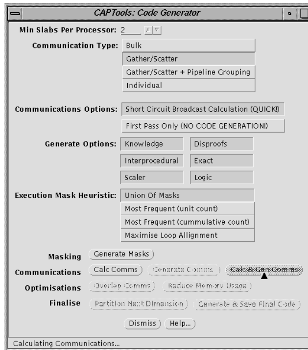
Figure T5-5: The Code Generator window for the final generation of message-passing code.
