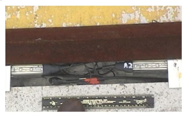
FIGURE 8. CONNECTION SPACE BETWEEN LED SECTIONS
