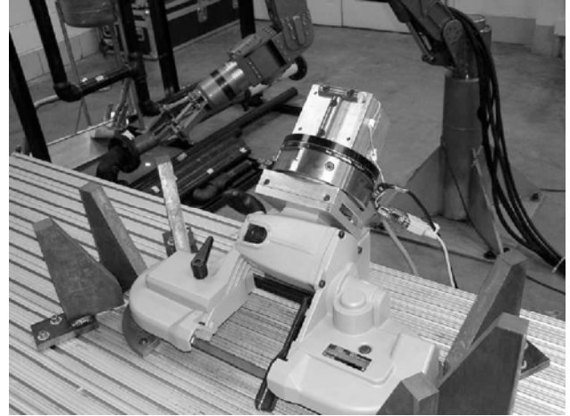
Fig. 7. Assembled band saw smart tool.
