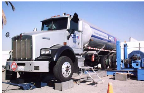
Figure 1. Tanker Truck Testing on the West Virginia University Transportable Chassis Dynamometer and Emissions Laboratory
