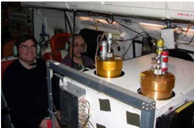
Figure 1. Jim Podolske of NASA/Ames and Tom Slate of NASA/Langley sit in front of the DAACOM/DLH instrument. This instrument makes extremely precise measurements of H_2O , CH_4 , CO , and N_2O .
