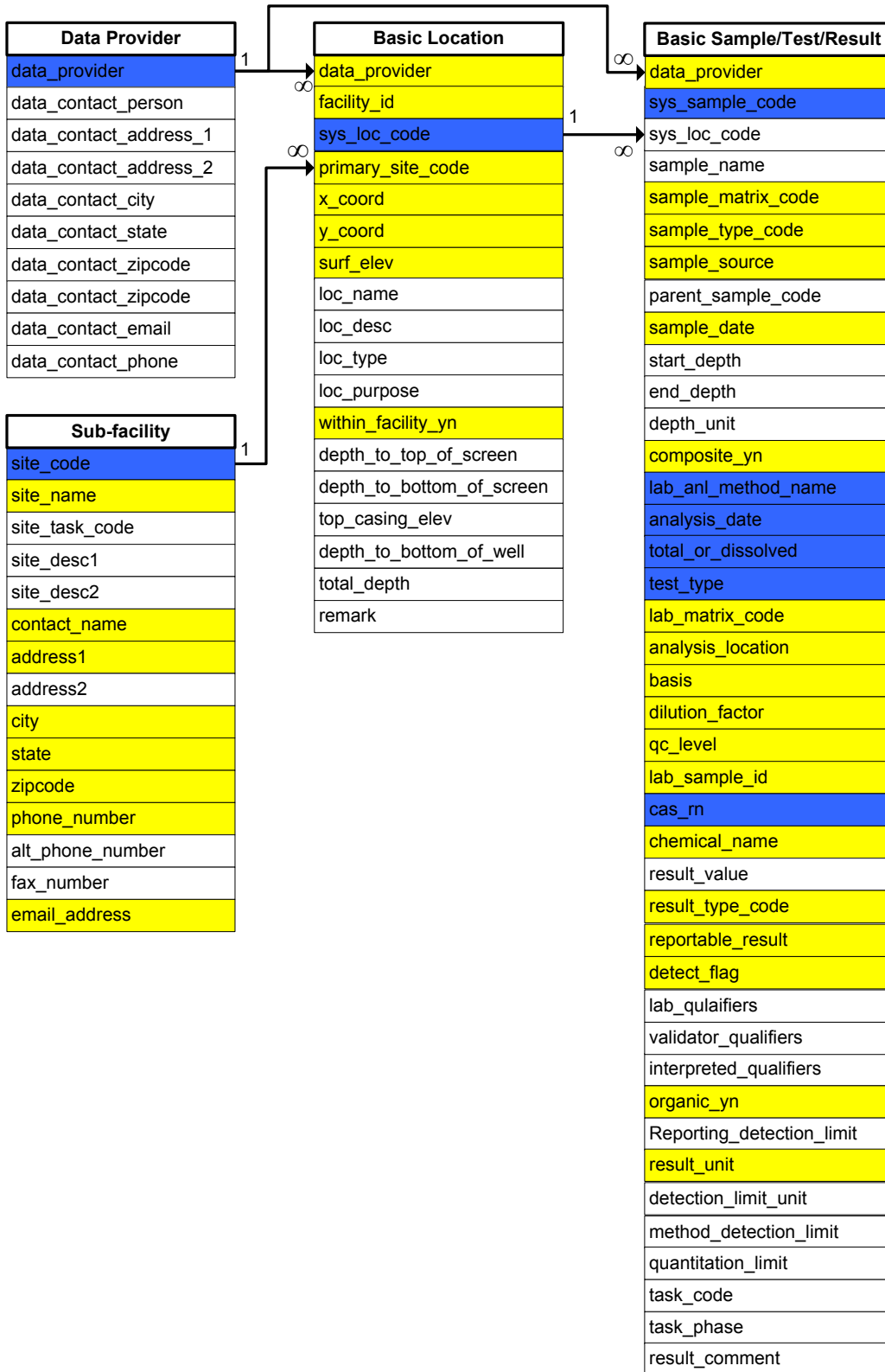
Figure 2-1 Relationships Between Basic EDD File Data Structures. Shaded fields are required to have data. Blue fields define row uniqueness for the specified file.
