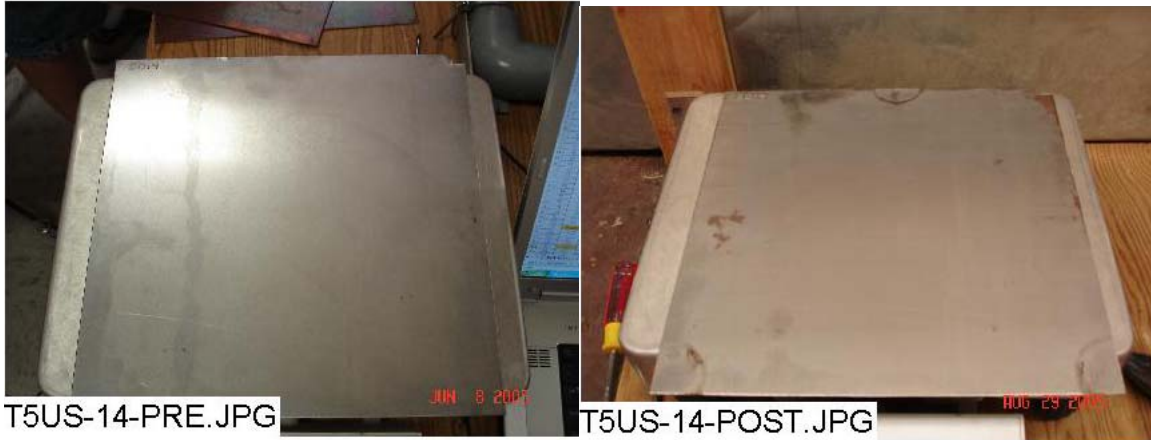
Figure 3-81. US-14 submerged, pre-test (left) and post-test (right).
