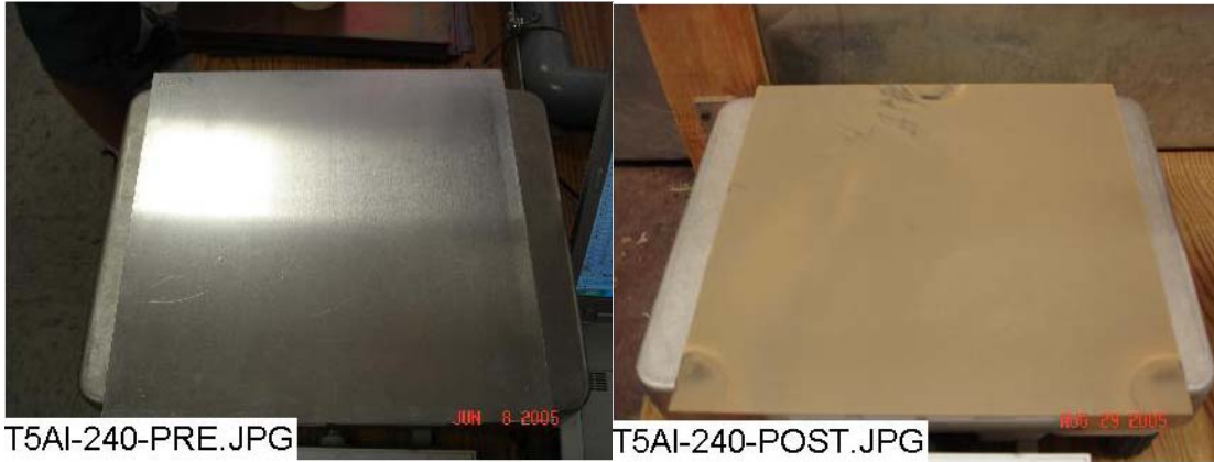
Figure 3-71. AI-240 submerged, pre-test (left) and post-test (right).
