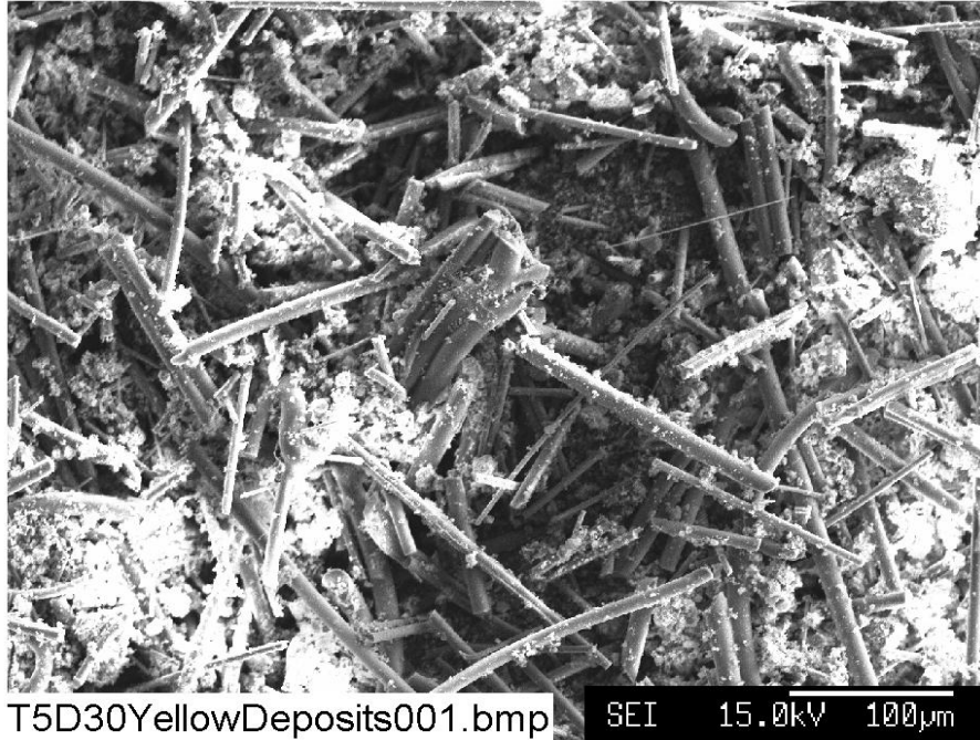
Figure 3-100. SEM image magnified 200 times for the Test #5, Day-30 fine yellow powder on the submerged rack.
