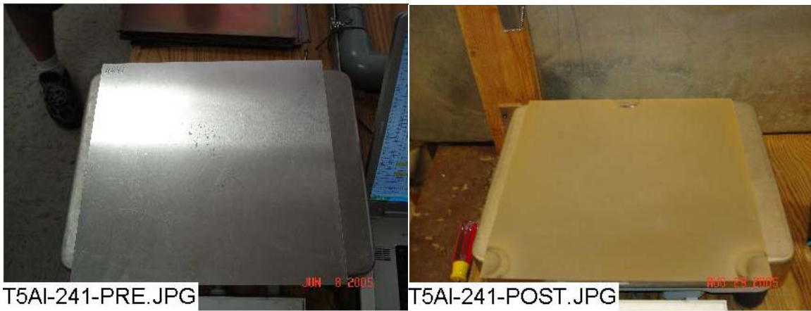
Figure 3-72. AI-241 submerged, pre-test (left) and post-test (right).
