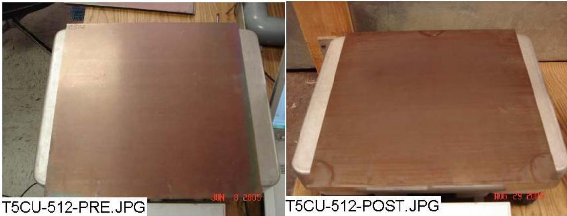
Figure 3-79. CU-512 submerged, pre-test (left) and post-test (right).
