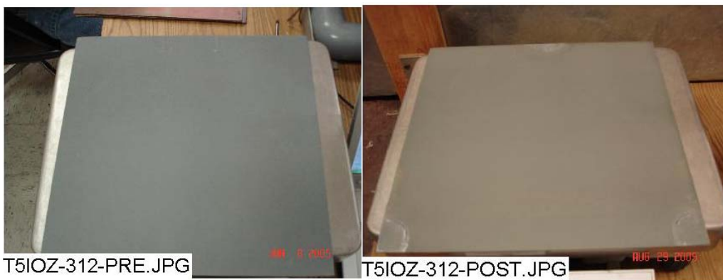
Figure 3-78. IOZ-312 submerged, pre-test (left) and post-test (right).
