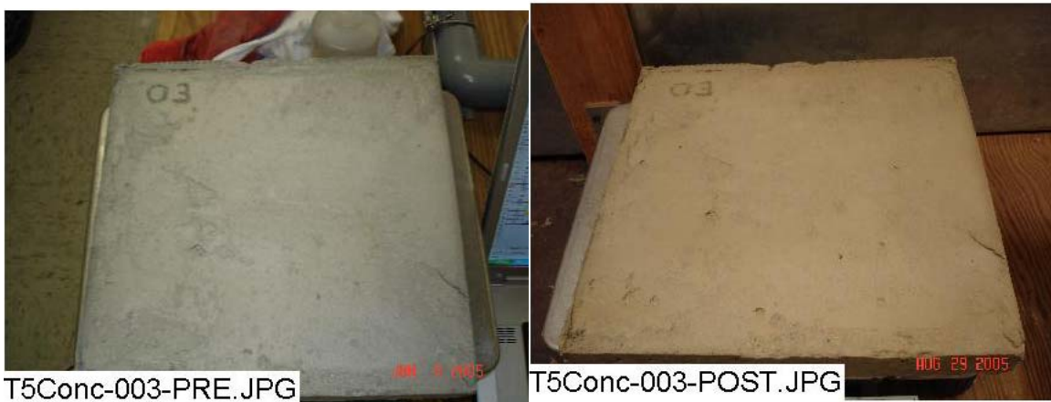
Figure 3-82. Conc-003 submerged, pre-test (left) and post-test (right).
