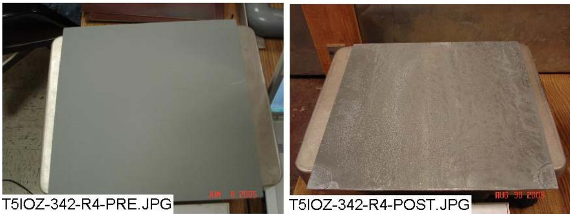
Figure 3-89. IOZ-342 unsubmerged, pre-test (left) and post-test (right).
