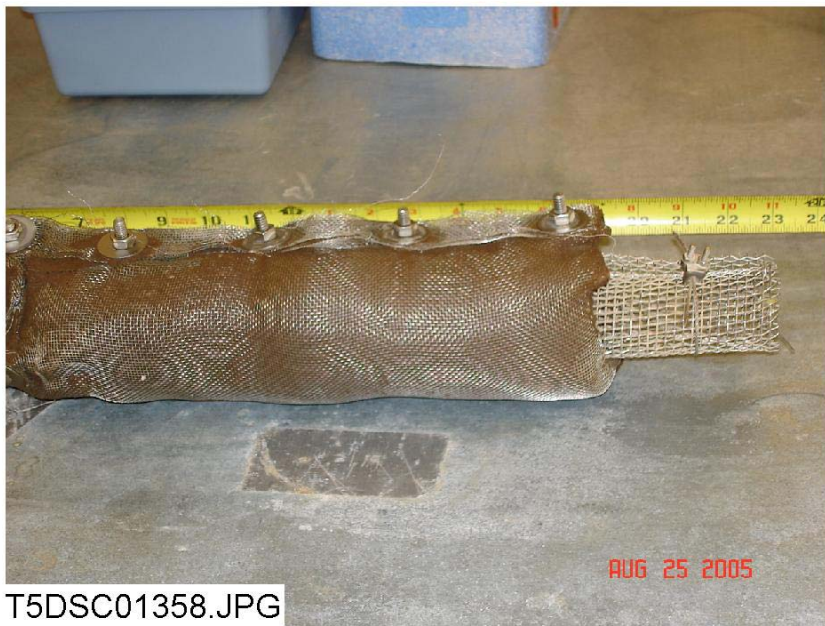
Figure 3-94. Drain collar removed from the tank bottom.
