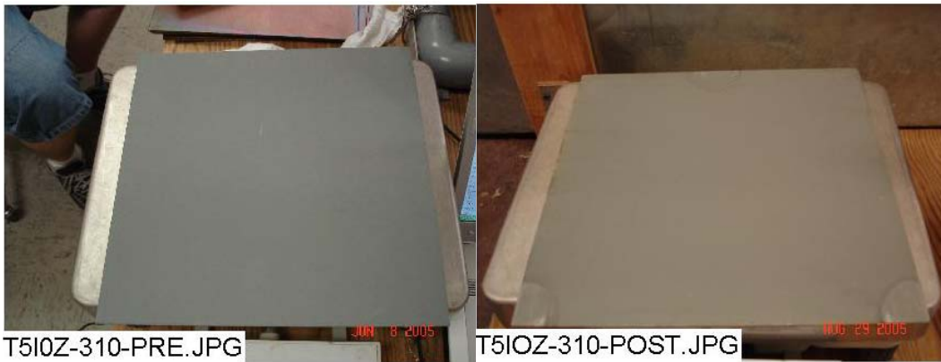
Figure 3-77. IOZ-310 submerged, pre-test (left) and post-test (right).
