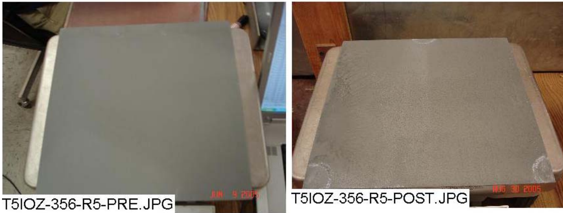
Figure 3-90. IOZ-356 unsubmerged, pre-test (left) and post-test (right).
