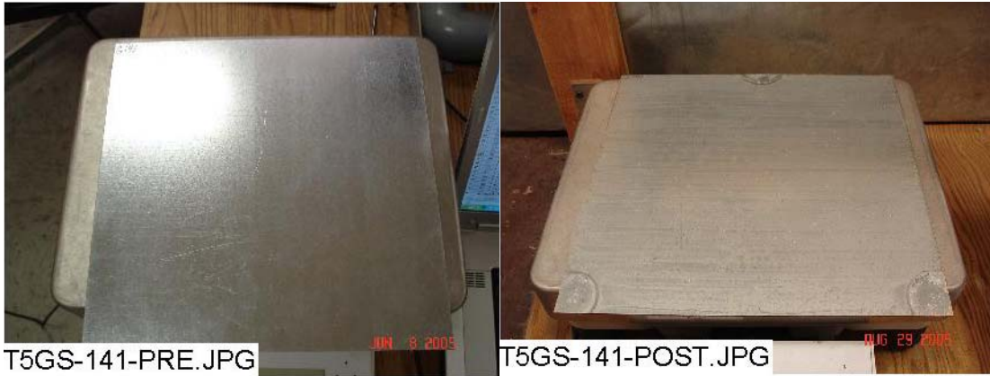
Figure 3-76. GS-141 submerged, pre-test (left) and post-test (right).
