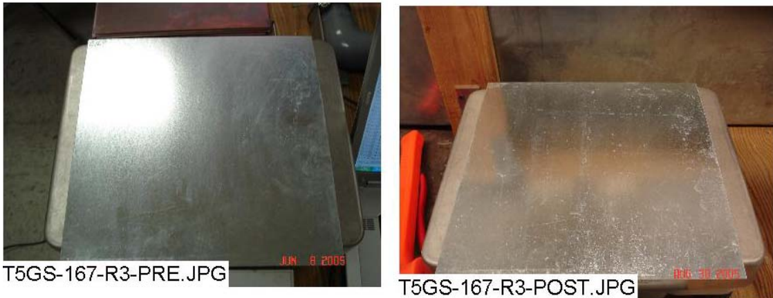
Figure 3-85. GS-167 unsubmerged, pre-test (left) and post-test (right).
