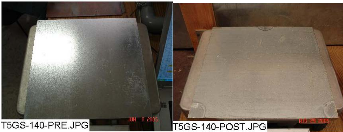
Figure 3-75. GS-140 submerged, pre-test (left) and post-test (right).
