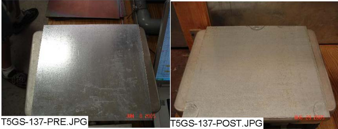
Figure 3-74. GS-137 submerged, pre-test (left) and post-test (right).
