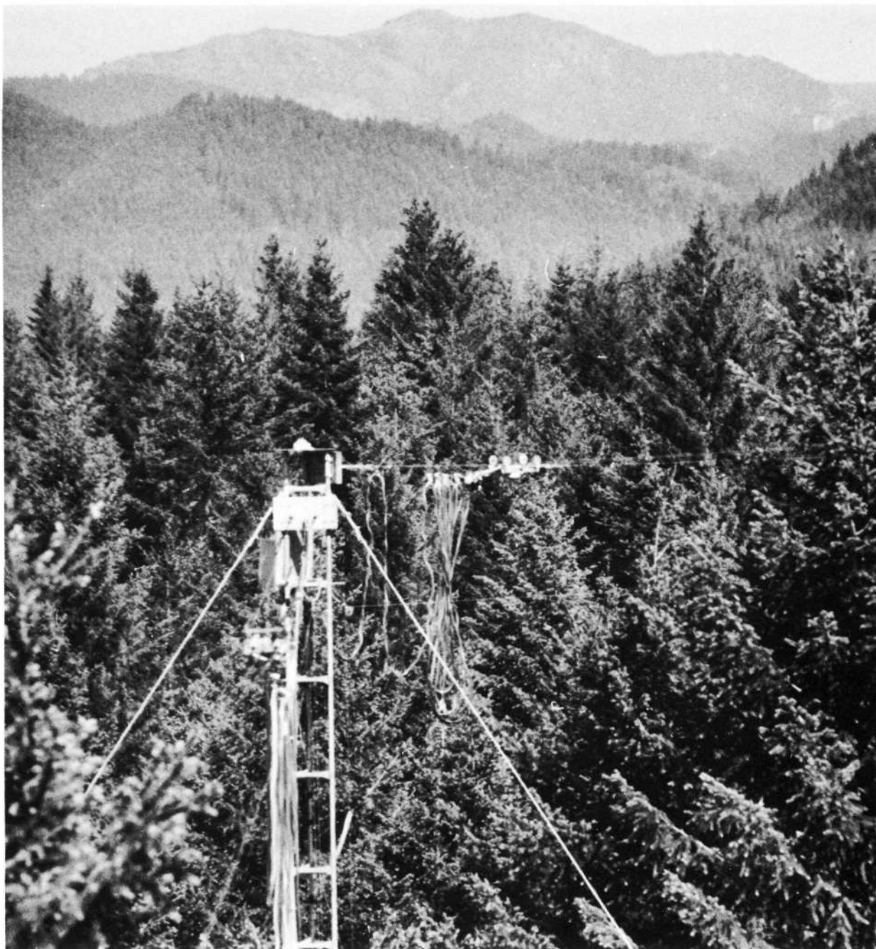
Figure 12B. Improved ground data instrumentation. Aerial tramway to collect solar radiation and emission data continuously over the trees.
