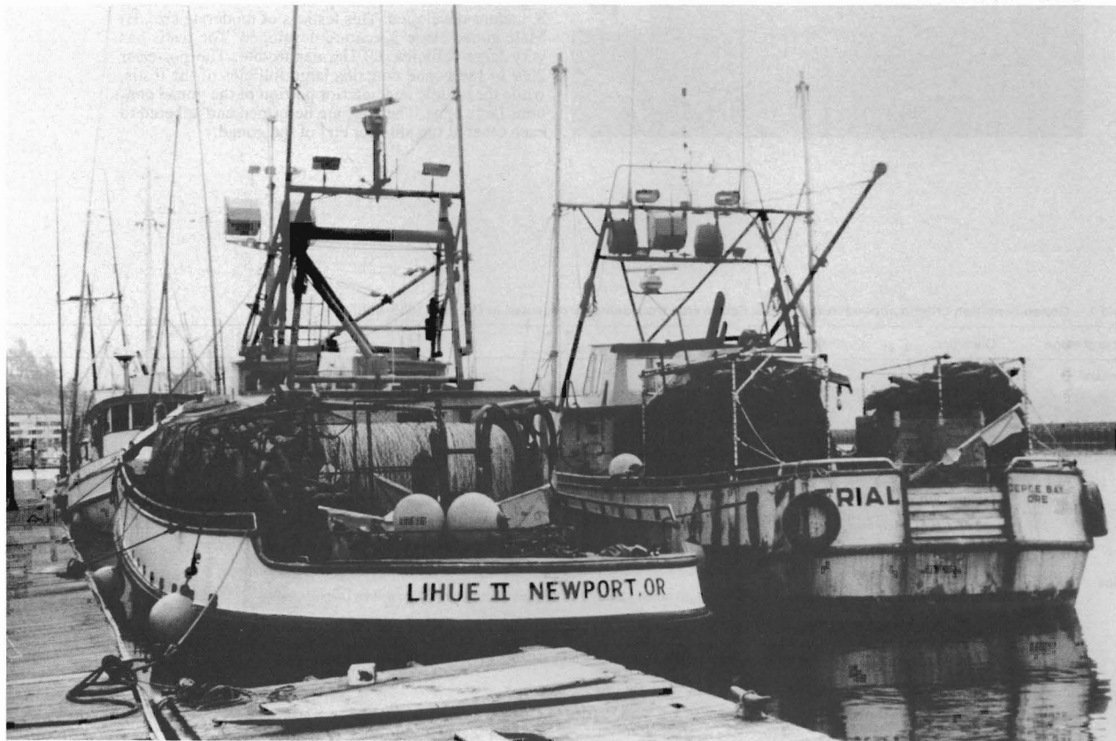
Figure 4.—F/V Lihue II and F/V Trial were two of the vessels that used the Korean traps for catching Pacific hagfish off Oregon in 1989. Fishing gear (traps, buoys, groundline, and flags) common to this fishery is on the back of the vessels.
