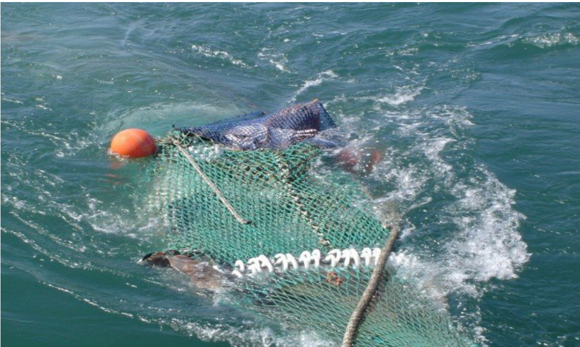
Figure 6. Photographs of the TED equipped trawl on haul-back showing the clogging by dogfish, skates and rays ahead of the TED grid.
