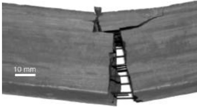
Figure 7. Photographs of the broken CSS steel wire reinforced concrete specimen after four-point bending test.
