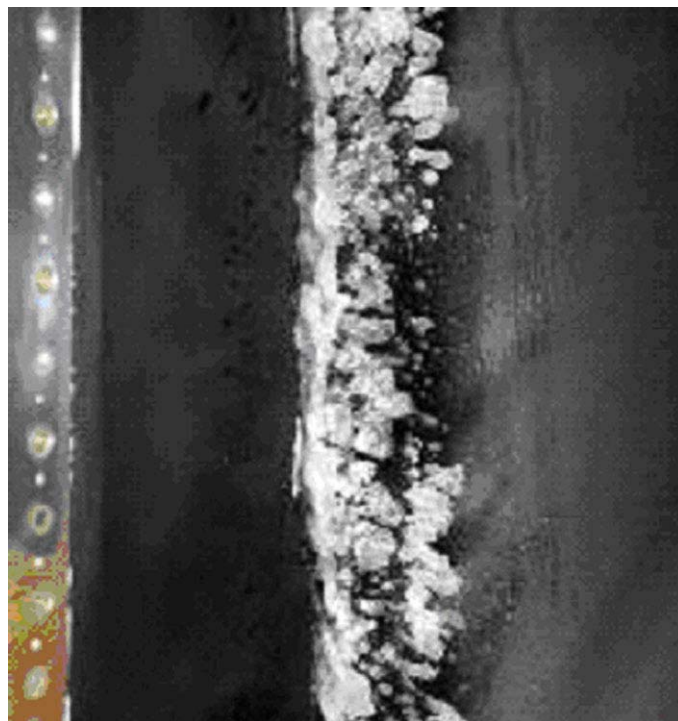
Figure 8. Close-Up Photograph (Pressure Surface) of a Warm-Hold SLD Runback Accretion After a 22.5-Minute Spray, Using the h, k_0, RHF Scaling Method (flow from left to right)
