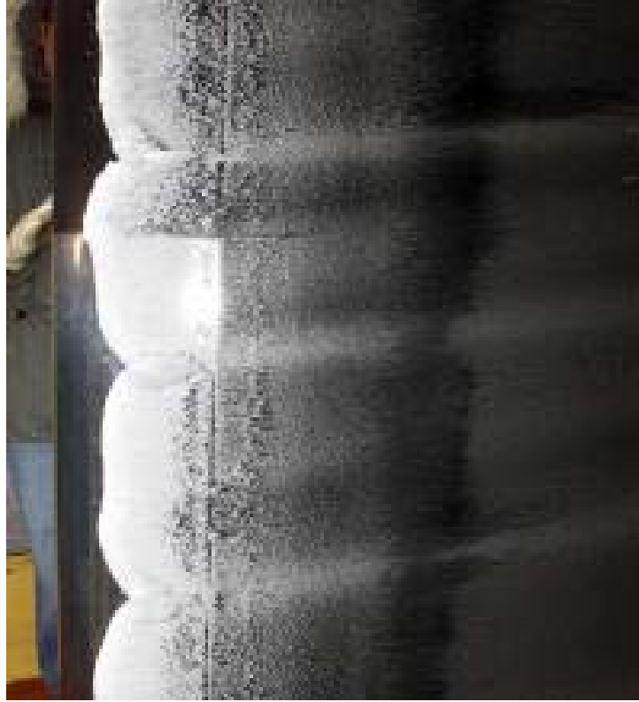
Figure 11. Overall Photograph (Pressure Surface) of a Cold-Hold Runback Accretion After an 8.6-Minute Spray, Using the h , k_0 , RHF Scaling Method (flow from left to right)
