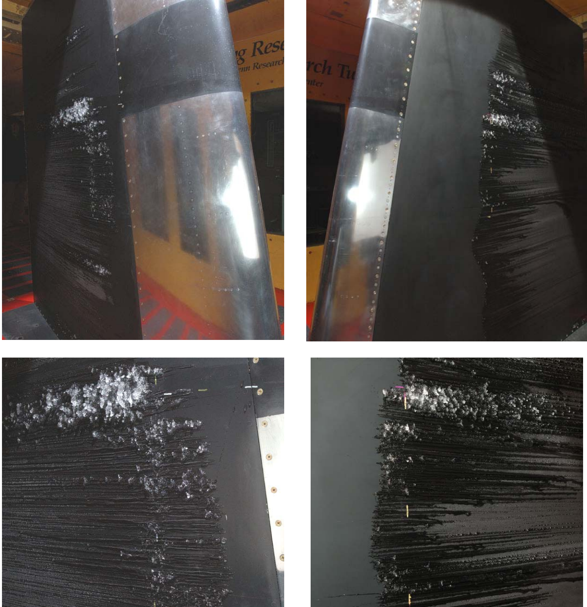
Figure B-3. Warm-Hold Run at a Total Temperature of 27.0°F. (The top shows the conditions for the run. Clockwise from the upper left are photographs showing the suction surface looking downstream, the pressure surface looking downstream, a close-up of the pressure surface, and a close-up of the suction surface.)
