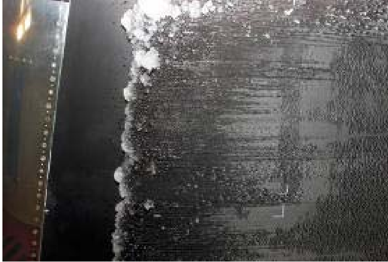
Figure 6. Overall Photograph (Pressure Surface) of a Warm-Hold Runback Accretion After a 22.5-Minute Spray, Using the h , k_0 , RHF Scaling Method (flow from left to right)
