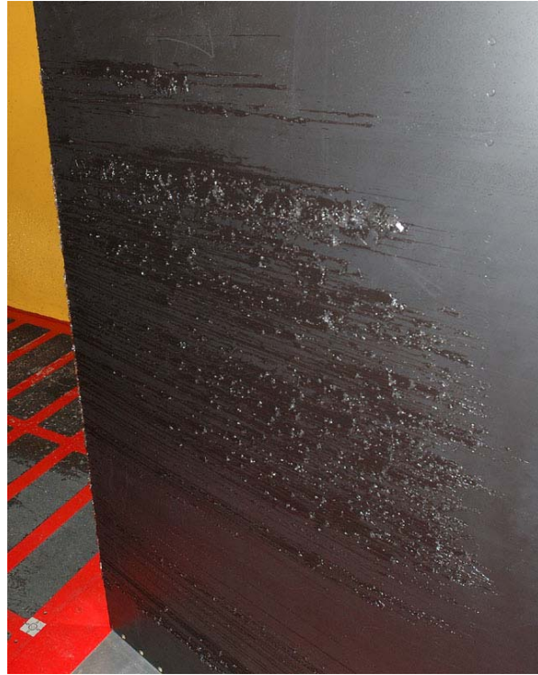
Figure 15. Photograph of the Suction Surface (Trailing-Edge Region) for the Warm-Hold Case With Matched Total Temperature (flow from right to left)
