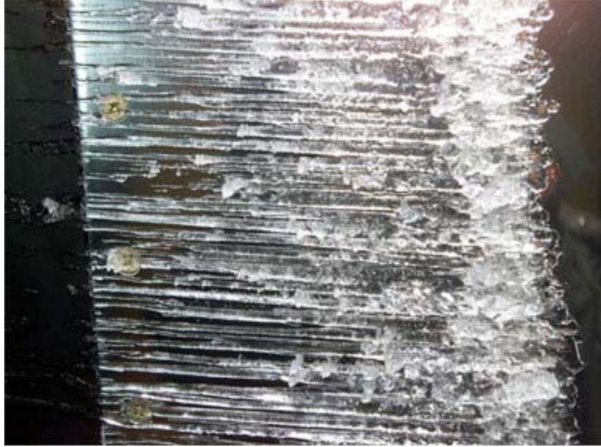
Figure 4. Close-Up Photograph (Suction Surface) of a Warm-Hold Runback Accretion After a 22.5-Minute Spray, Using the h, k_0 , RHF Scaling Method (flow from right to left)
