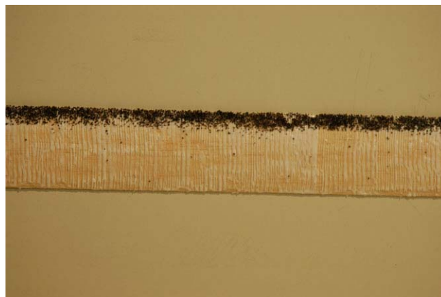
Figure 22. Photograph of Suction Surface 3-D Ice Shape Simulation for Warm-Hold Case
