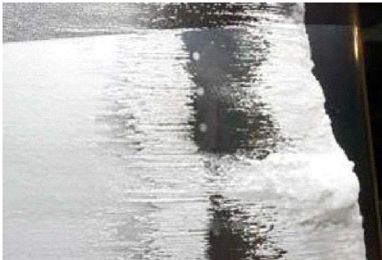
Figure 10. Close-Up Photograph (Suction Surface) of a Cold-Hold Runback Accretion After an 8.6-Minute Spray, Using the h , k_0 , RHF Scaling Method (flow from right to left)
