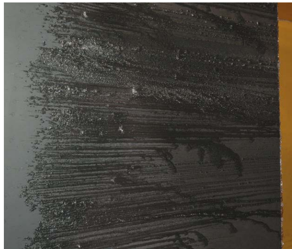
Figure B-4. Warm-Hold run at a Total Temperature of 28.5°F. (The top shows the conditions for the run. Clockwise from the upper left are photographs showing the suction surface looking downstream, the pressure surface looking downstream, a close-up of the pressure surface, and a close-up of the suction surface.)
