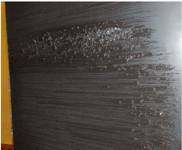
Figure B-4. Warm-Hold run at a Total Temperature of 28.5°F. (The top shows the conditions for the run. Clockwise from the upper left are photographs showing the suction surface looking downstream, the pressure surface looking downstream, a close-up of the pressure surface, and a close-up of the suction surface.)
