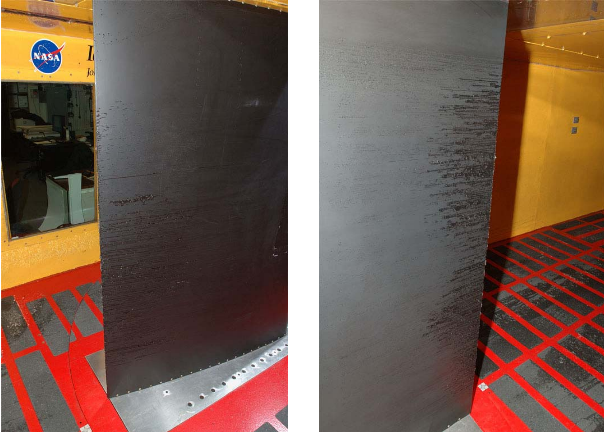
Figure B-5. Warm-Hold Run at a Total Temperature of 29.9°F. (The top shows the conditions for the run. At left is a photograph of the suction surface trailing edge, and at right is a photograph of the pressure-surface trailing edge.)
