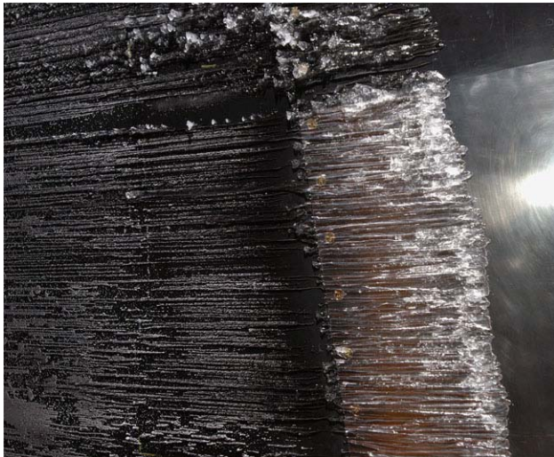
Figure B-1. Warm-Hold Run at a Total Temperature of 23.0°F. (The top shows the conditions for the run. Clockwise from the upper left are photographs showing the suction surface looking downstream, the pressure surface looking downstream, a close-up of the pressure surface, and a close-up of the suction surface.)
