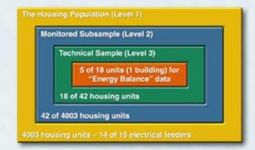
For ORNL's evaluation of the Fort Polk project, data were collected to show electricity consumption per feeder (Level 1), per apartment (Level 2), and per water heater and heating/ cooling system (Level 3). "Energy balance" data were collected from one building.
