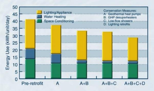
Impact of retrofits on electricity use for space conditioning, water heating, and lighting and appliances (Feeder I).
