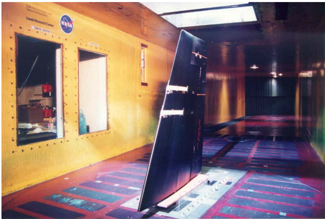
Figure 4: Illustration of wing blotter strip installation.
