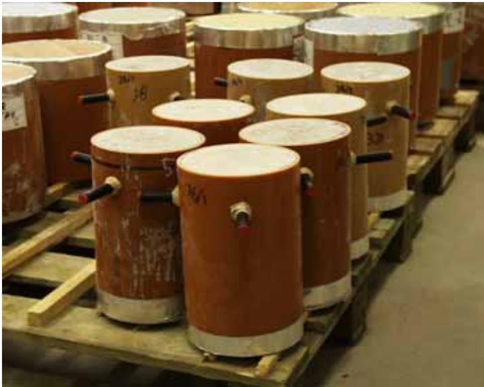
Figure 3.5 - RH was measured with the RH-sensor Vaisala HMP 44 in plastic pipes that were drilled into the specimen at 20% depth of the length, i.e. 50 mm from the end.
