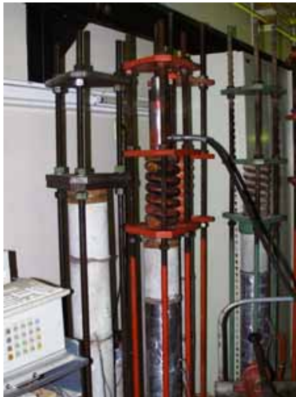
Figure 2 - Basic creep specimens loaded with a hydraulic jack in the center spring-loaded frame
