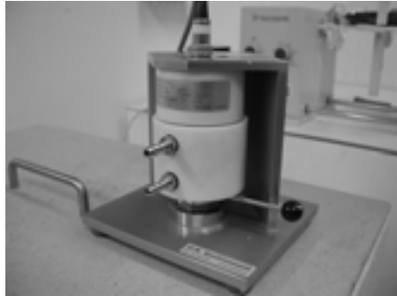
Figure 1 – Rotronic Hygroscope DT station for measurements of autogenous relative humidity of cement pastes.
