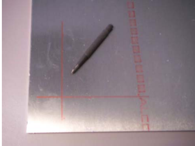
Figure 8 : Mark and punch the stake holes
