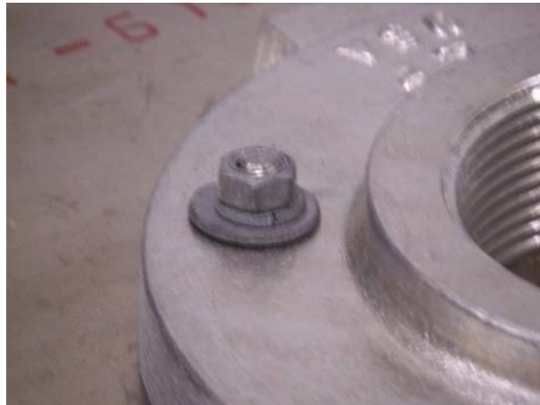
Figure 9 : Mounting the flange to the plate
