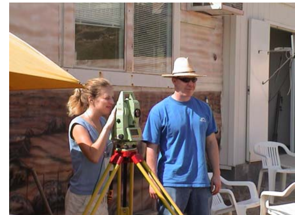
Measuring Ground Truth using Total Station
