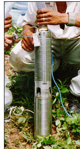
Fig. 5: Submersible centrifugal pump
