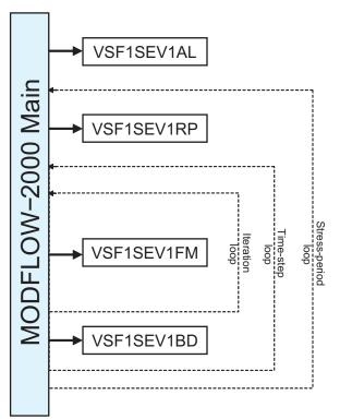
**Figure 7.** Subroutines used by the Surface Evaporation (SEV1) Package. A typical simulation proceeds from top to bottom.
