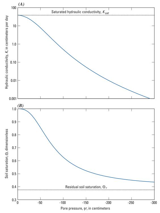
**Figure 2.** Soil characteristic functions for (*A*) hydraulic conductivity,  $K(\psi)$ , and (*B*) soil saturation,  $\Theta(\psi)$ , as a function of pore-water pressure. This soil type is used in simulation example case 2.
