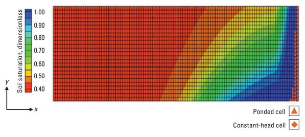
Figure 24. Plan view of simulated soil saturations and ponded cells for day 299.
