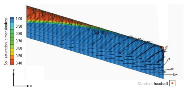
**Figure 23.** Longitudinal cross-section view showing simulated soil saturations and flow vectors along grid row 1 at the start of day 299. Note that the flow vectors are scaled relative to magnitude, and the *z* scale is exaggerated 10 times.
