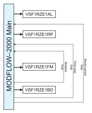
**Figure 8.** Subroutines used by the Root Zone Evapotranspiration (RZE1) Package. A typical simulation proceeds from top to bottom.
