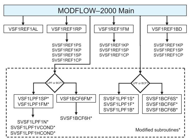
**Figure 3.** Subroutines used by the Richards' Equation Flow (REF1) Package. A typical simulation proceeds from left to right. Existing subroutines that have been modified are contained in a dashed box.
