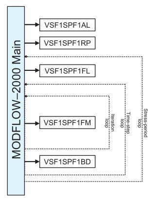
**Figure 4.** Subroutines used by the Seepage Face (SPF1) Package. A typical simulation proceeds from top to bottom.
