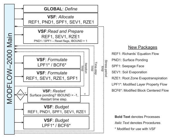
**Figure 1.** Structure of the Variably Saturated Flow (VSF) Process and its interactions with MODFLOW–2000. Simulations are controlled by MODFLOW's main program (left) and proceed from top to bottom, cycling through the nested iteration, time-step, and stress-period loops.
