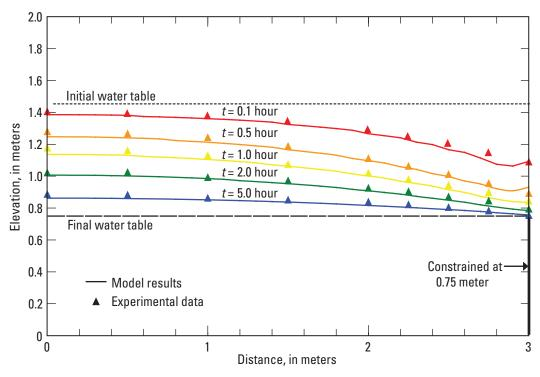
**Figure 14.** Modeled water-table positions for two-dimensional drainage study plotted in relation to experimental data of Vauclin and others (1975).
