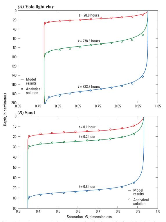
**Figure 11.** Comparison between simulated water saturation ( $\Theta$ ) profiles and Phillip's analytical solution for one-dimensional, constant-head infiltration in (*A*) Yolo light clay and (*B*) sand.
