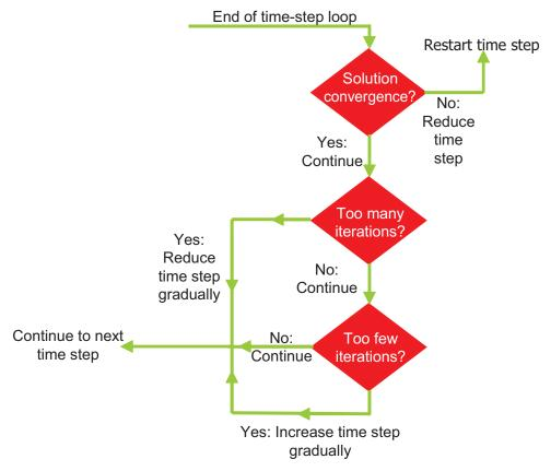
Figure 9. Algorithm for the Adaptive Time-Stepping (ATS1) Package.
