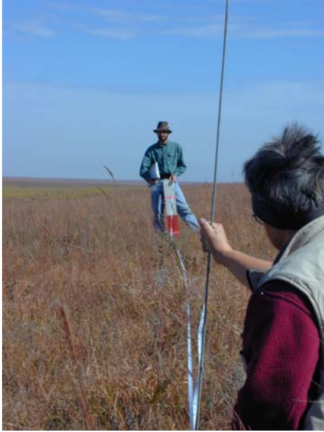
Figure 5.1. Conducting the horizontal cover measurements using profile board and sighting pole.
