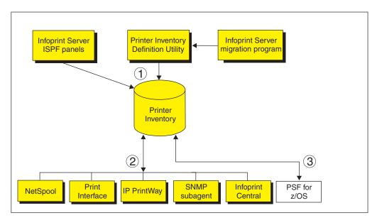
Figure 2. Printer Inventory Manager system diagram
