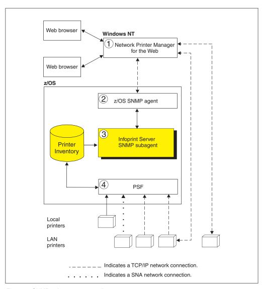
Figure 9. SNMP subagent system diagram
