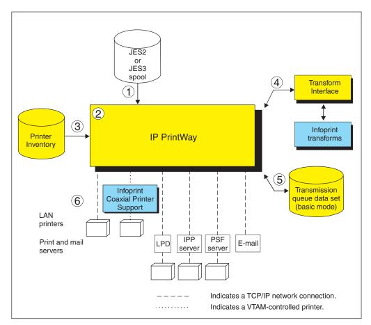
Figure 7. IP PrintWay system diagram
