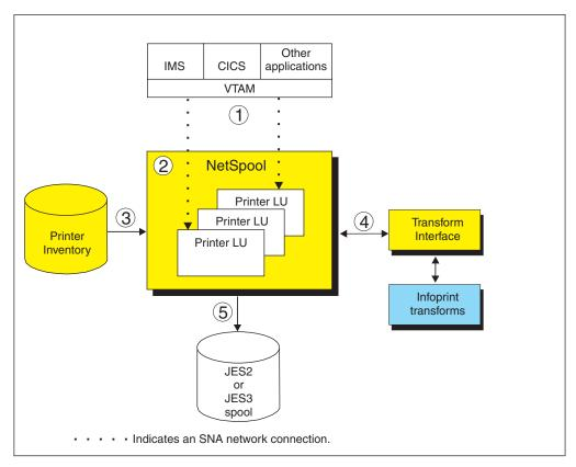
Figure 6. NetSpool system diagram
