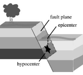
called the *fault* or *fault plane*. The location below the earth's surface where the earthquake starts is called the *hypocenter*, and the location directly above it on the surface of the earth is called the *epicenter*.
