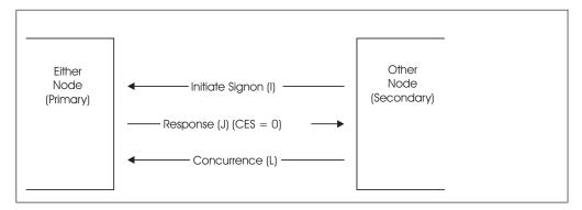
Figure 31. Secondary Trunk Connection
