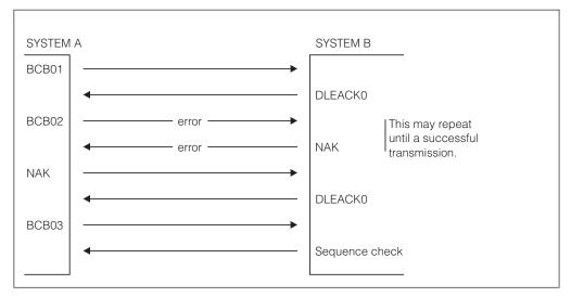
Figure 16. Results of Not Transmitting Null Records.
