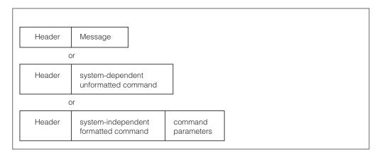
Figure 7. Format of an NMR
