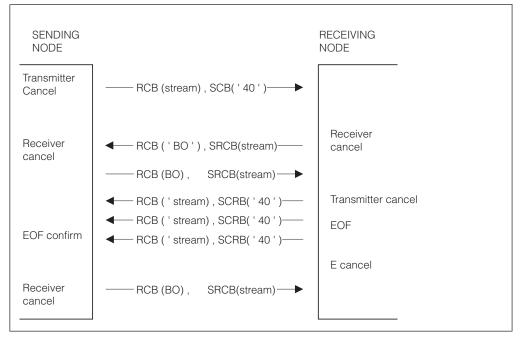
Figure 26. Sending Node Initiates Stream End
