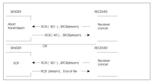
Figure 27. Receiving Node Initiates Stream End
