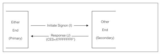
Figure 28. Connection Protocols used by the Non-Path Manager Nodes
