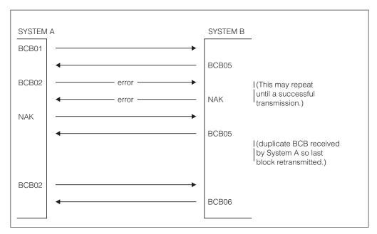
Figure 17. Correct Recovery with Null Records
