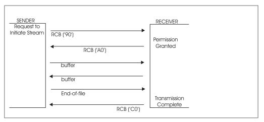
Figure 24. Protocols Used to Transmit a Stream
