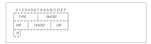
Figure 59. Format for the control record
