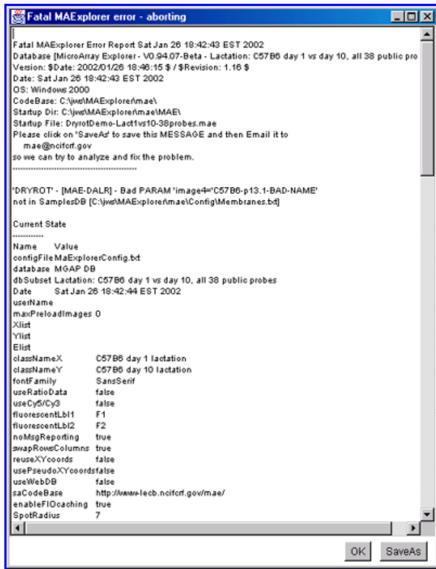
Figure 4.4 Example of a fatal Dryrot Error window. This may occur for a variety of reasons. This window lists the main reason and also lists some of the MAExplorer state information. If you wish, you may save this window (press the "SaveAs" button) and mail it to us. We may try to correct the problem in the next release if it is a problem with MAExplorer. Alternatively, it could be a user data error.
