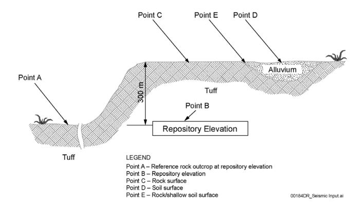
Figure 6.1.3-1. Seismic Design Input Locations
