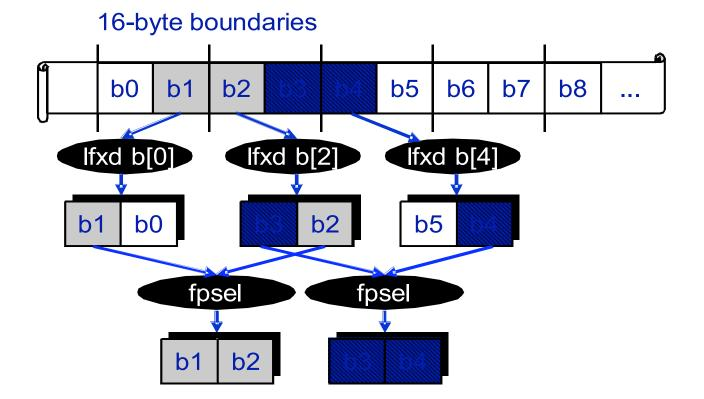
1 misaligned-quad load costs on avg. 1 aligned-quad cross-loads + 1 sele
