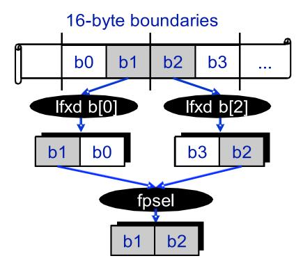
1 misaligned-quad load costs 2 aligned-quad cross-loads + 1 select
