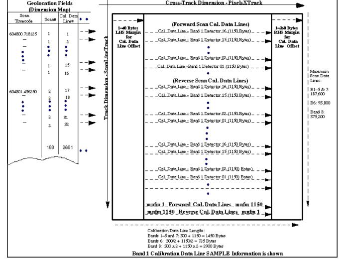
Figure 2-5. Calibration Data File - ECS-HDF Swath Overview
