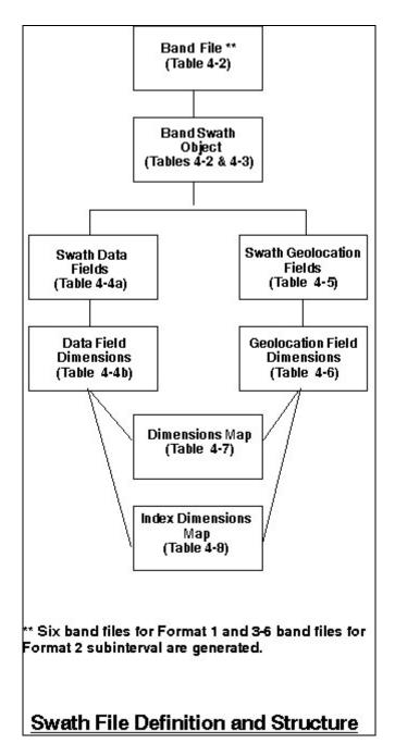
Figure 2-1. Band Data File - HDF-EOS Swath Structure
