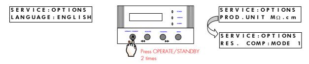
Press the CLEANING Keypad Button twice to change from MODE 1 to OFF. The Resistivity Temperature Compensation will now be off.
