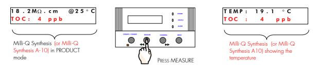
The temperature will be displayed for about 10 seconds. The LCD will return to the resistivity display.
