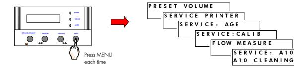
**WAIT.** Do not press the Keypad. The A10 CLEANING mode will start automatically after 5 seconds. The 60 minute timer will be shown.
