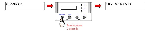
Press the MENU Keypad button for about 2 seconds. The LCD will change as shown here:
