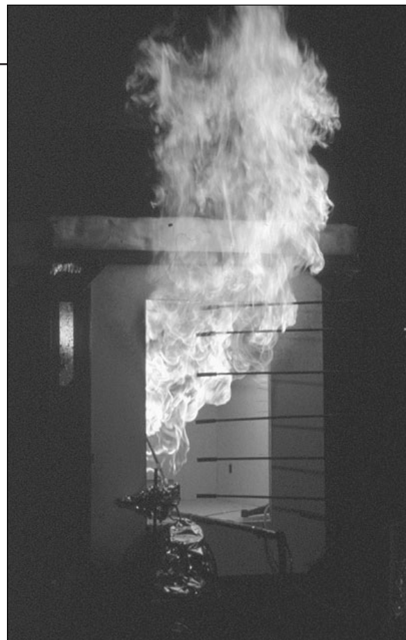
A scale model experiment used to investigate carbon monoxide formation during underventilated burning within an enclosure.
