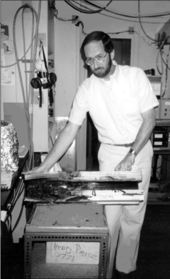
Thomas Ohlemiller, chemical engineer, examines the results of an experiment to characterize the smoldering combustion of blown-in cellulosic insulation in attic spaces.
