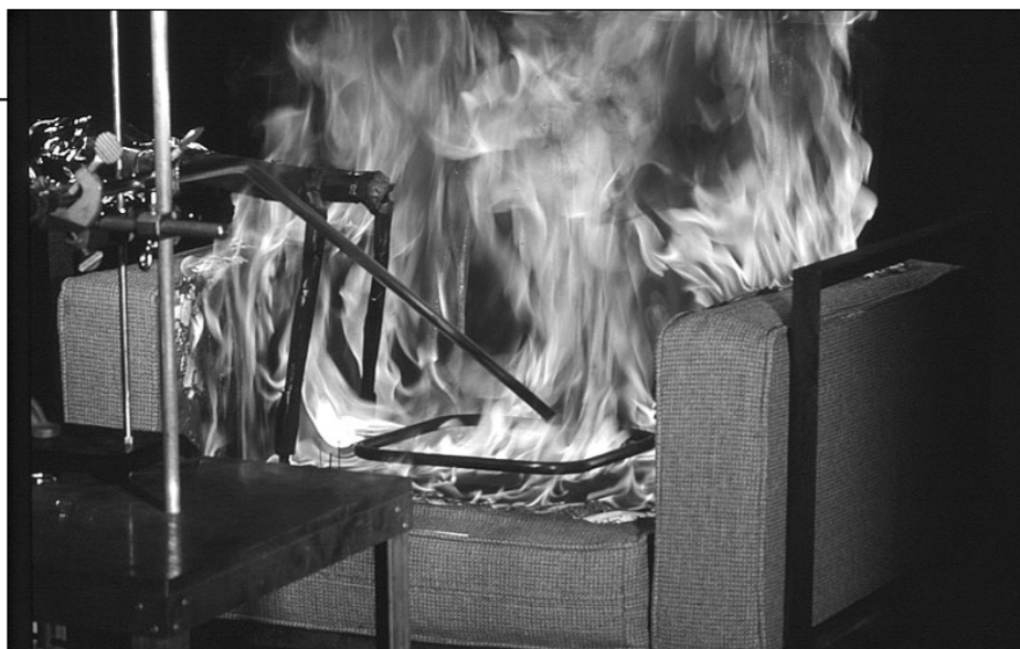
A furniture mock-up subjected to the California Technical Bulletin 113 gas flame igniter that was developed at NIST. To the left of the burner are two heat flux gages measuring the energy feedback from the flames.
