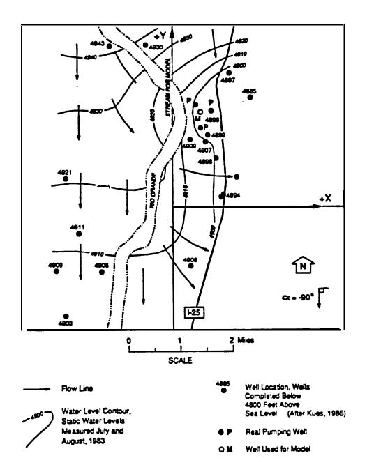
From Newsom and Wilson, 1988. P's represent actual municipal wells, and M represents the imaginary model well. The x and y coordinate axis used by MWCAP are superimposed upon the general flow field.
