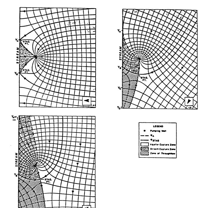
zone boundary becomes tangential to the stream boundary, it is necessary to identify point A (the critical tangent point). Once this point is located two additional panicles can be released from its neighborhood to trace the boundary segments of the capture zone. The location of A can be determined using the following expression of stream function derived from (B.15):
