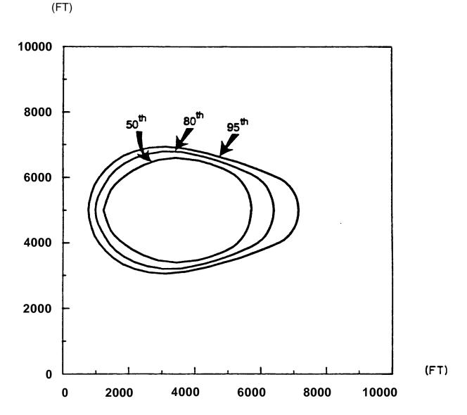
To illustrate the cause of the pear shapes more clearly, two additional capture zones were delineated using MWCAP (recall. that much of the MONTEC module is based upon the MWCAP module). The smallest and the largest transmissivity values generated during the 1,000 MONTEC iterations were used as input for the first and second MWCAP runs respectively. The values were extracted from the standard MONTEC output file CAPTUR.VAR. All of the input parameters for each MWCAP run arc presented m Table 9.3.
