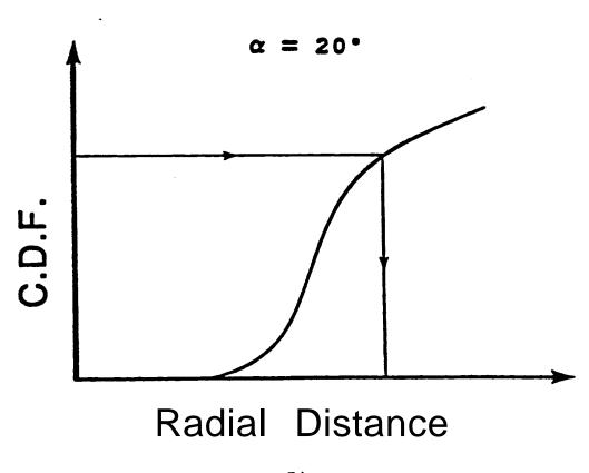
Once N capture zones have been generated by MONTEC, the N distances saved for each radial line arc sorted into ascending order. The resulting tabulation is the experimental cumulative distribution function (CDF) for each line. A sample CDF, which corresponds to the radial line defined by  $\alpha_i$  in Figure 9.1a is shown in Figure 9.1b.
