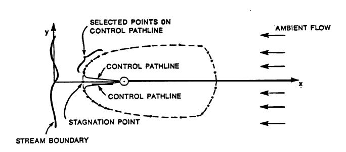
Figure B.7 Schematic Description of the Procedure Used to Locate the Capping **Boundary of a Hybrid Capture Zone**
