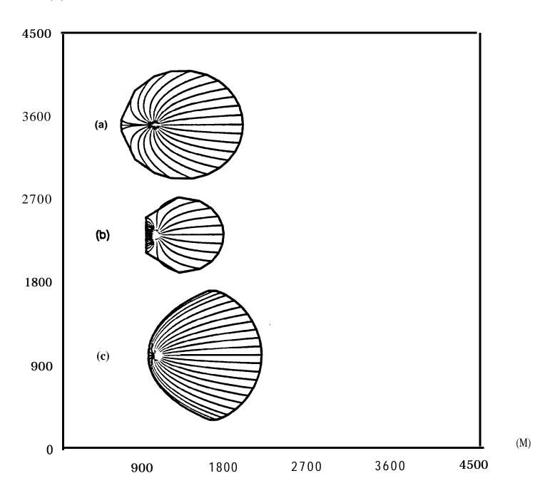
flow within **the** aquifer. The area enclosed by the capture zone that intercepts the stream is smaller than the other two because the stream boundary, in addition to the ambient ground-water flow, acts as a source of water to the well.
