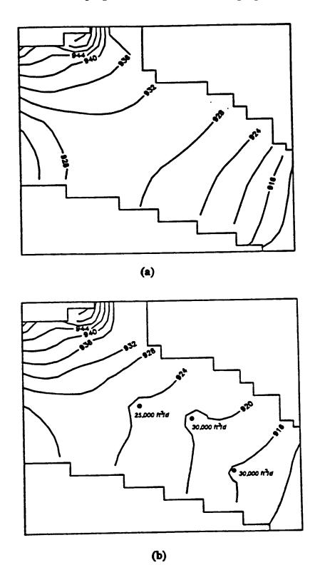
Once the head field for the second simulation was obtained using MODFLOW, the WHPA model was applied to delineate the 5-year capture zones for the three pumping wells. The required input for the GPTRAC numerical option is provided in Table 8.4, and the delineated capture zones are presented in Figure 8.10. The capture zones for this example are very complex due to the aquifer heterogeneities and well interference effects.
