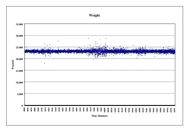
Figure 4.6. Rear axle weight measured during the selected 2-hour time period.
