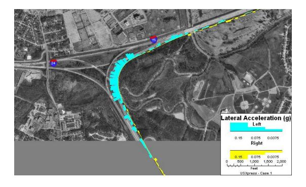
Figure 4.3. Truck trajectory on curve at junction of I-24/I-75 near Chattanooga, Tennessee.
