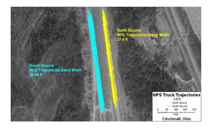
Figure 4.20. North-bound and south-bound, I-275, pre-May 1, 2001, truck trajectories measured near Cincinnati, Ohio. Note: band widths = 27 feet (north-bound) and 39 feet (south-bound).
