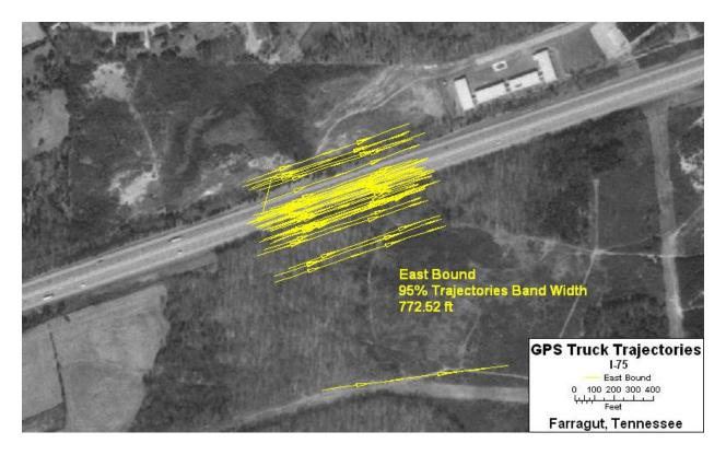
Figure 4.18. East-bound, I-75, pre-May 1, 2001, truck trajectories, measured near Knoxville, Tennessee. Note: band width = 773 feet.
