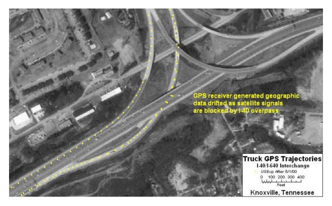
Figure 4.21. North-bound and south-bound, post May 1, 2001, truck trajectories, measured near Knoxville, Tennessee. Note the drift when signals were blocked by the overpass.
