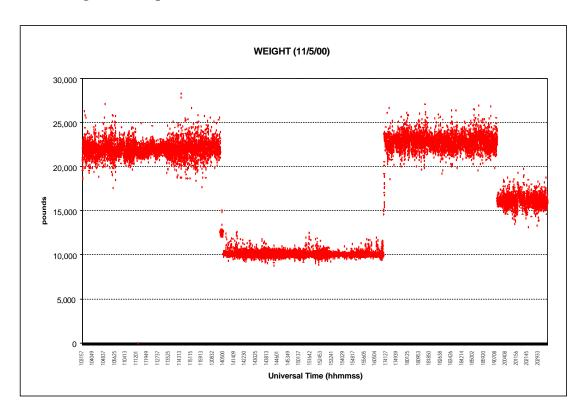
Figure 4.16. Weight measured on November 5, 2000, for a Praxair truck.
