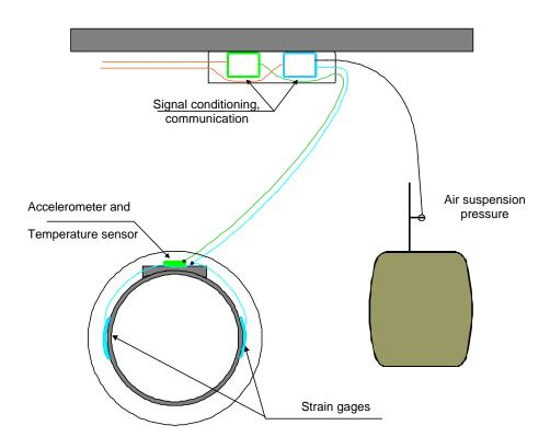
Figure 2.1. Axle sensors and signal conditioners.
