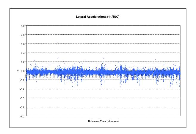
Figure 4.17. Lateral acceleration measured on November 5, 2000, for a Praxair truck.
