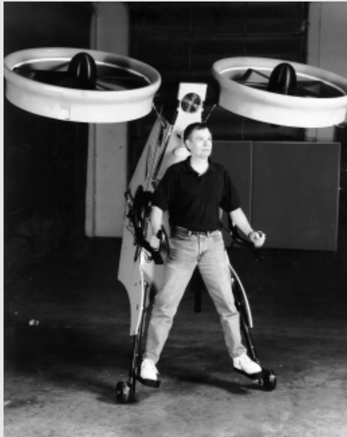
Michael Moshier, founder and CEO of Millennium Jet, Inc., Santa Clara, CA, demonstrates the Solo Trek Exo-Skeletor Flying Vehicle, a one-person air scooter, developed by Millennium Jet Inc. NASA Ames signed a Non-Reimbursable Space Act Agreement with Millennium Jet to develop the air scooter.
