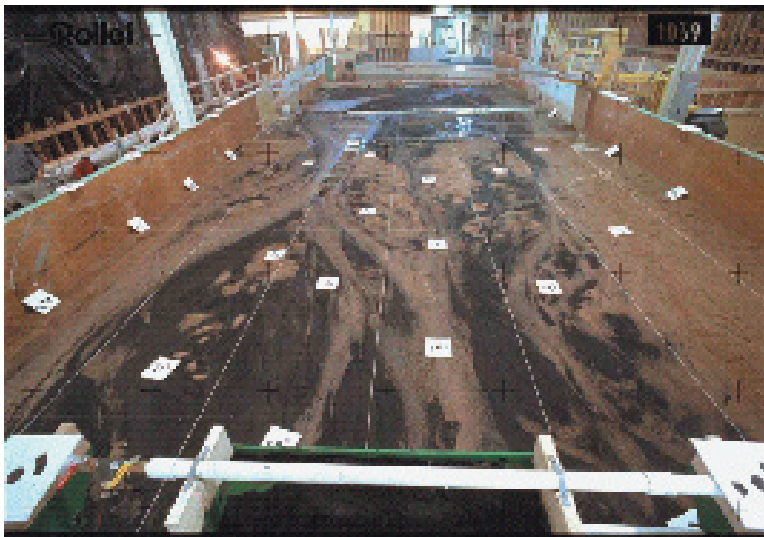
Coded targets set up on the Rio Grande model that was used as a pilot in 2005 to test detailed surface measurement.
