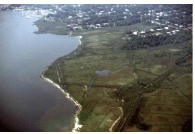
Figure 5. Aerial photo of grid ditching in Long Island tidal wetlands.
