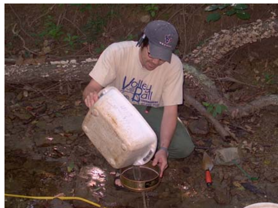
Figure 4-16 Sample elutriation in the wash basin and pouring invertebrates and fine detritus into the sieve.
