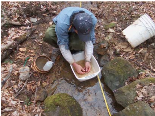
Figure 4-14 Scrubbing attached invertebrates off the coarse surface substrate in the wash basin (or sieve).
