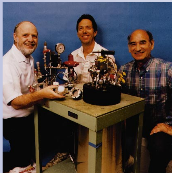
Pictured with the injection molding apparatus for rapid production of silica aerogels are, from left to right, Larry Hrubesh, John Poco, and Paul Coronado.
