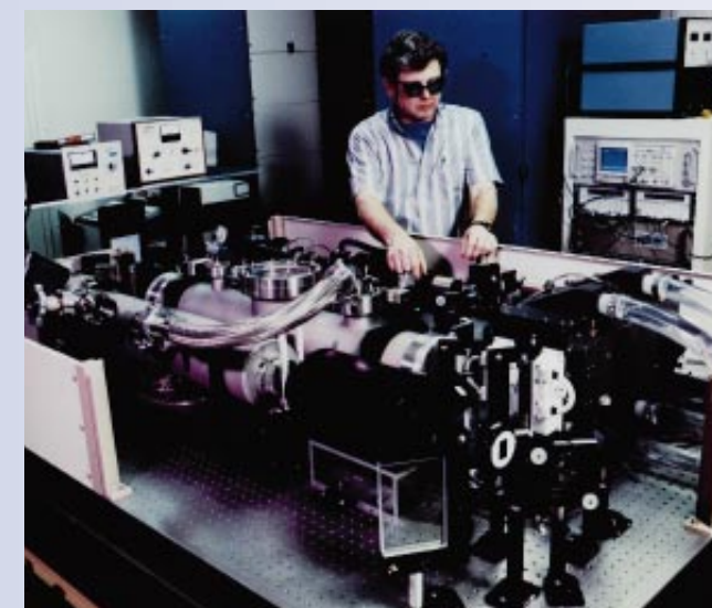
Electrooptics technician James Wintemute completes final alignment of a packaged laser system. Several of these systems have been installed and are in use, one of them at Kennedy Space Center in Florida, where it will be used to illuminate rocket launches.
