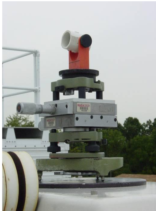
Close View Translation Stage and Prism on Trivet Plate
