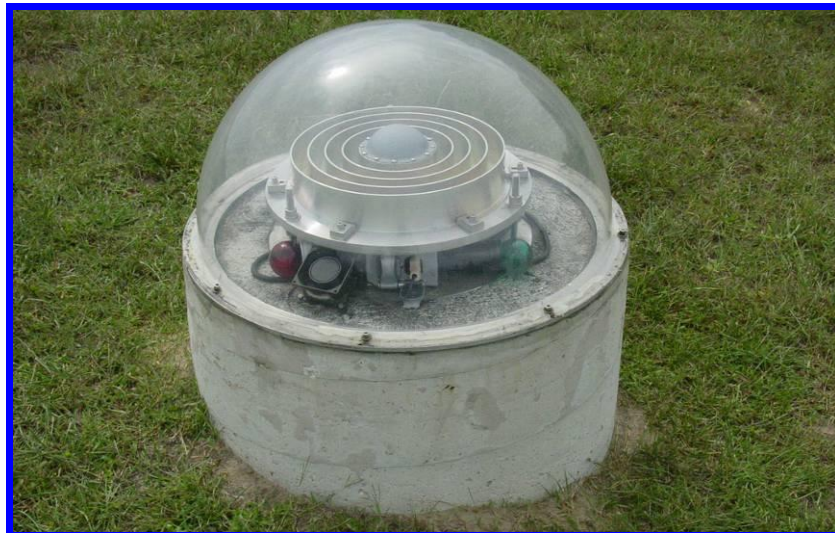
Figure 3. GPS GODE antenna on pier monument
