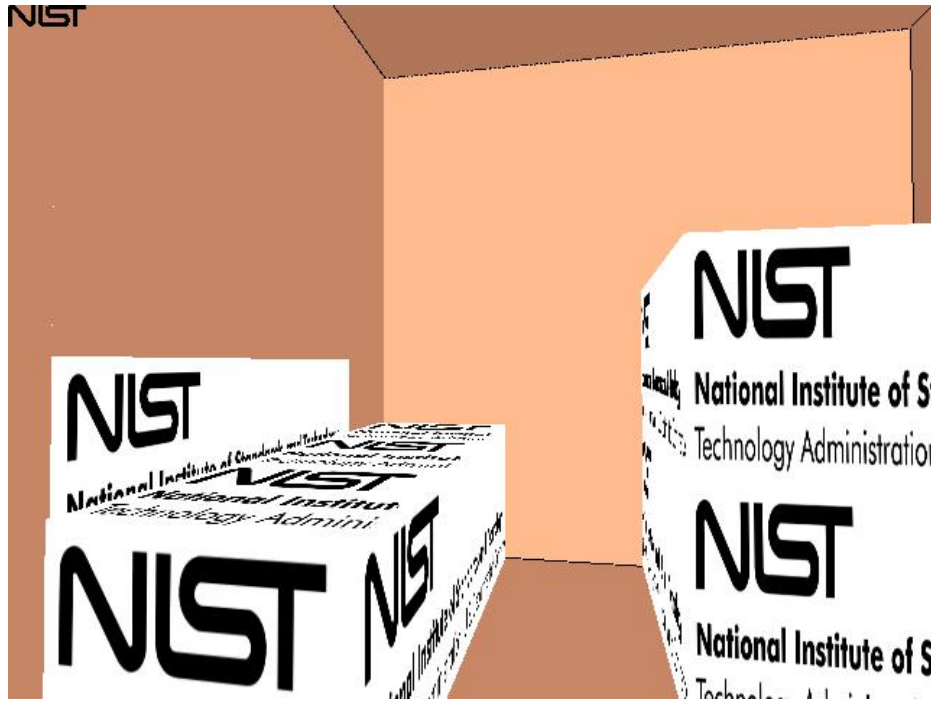
Figure 4.11: Texture map example. The same texture was applied to two different blockages and a vent (with different widths) by assigning different TEXTURE_WIDTH parameters in the input file.
