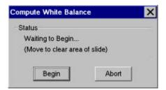
5. Click on the Begin button to start the calculation. The Compute White Balance window displays the status message **Computing white balance values**. You should hear a series of clicks as the camera samples the light.
