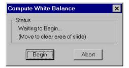
5. Click on the Begin button to start the calculation. The Compute White Balance window displays the status message **Computing white balance values**. You should hear a series of clicks as the camera samples the light.
