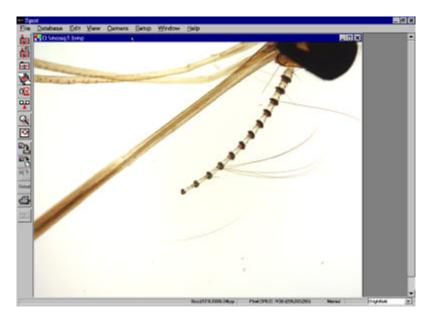
The image captured in the above diagram is off-center. Using the Frame option, you can adjust the position of the image without having to look through the microscope, recapture the image, and determine if it displays correctly. The Frame option enables you to adjust the specimen's position using the on-screen image as a reference. The Frame option can also be used before you have captured an image.
