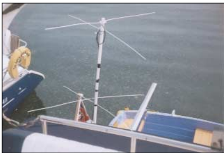
Figure 7 - The APT antenna mounted on Colin Cox's boat while sailing the Solent.
