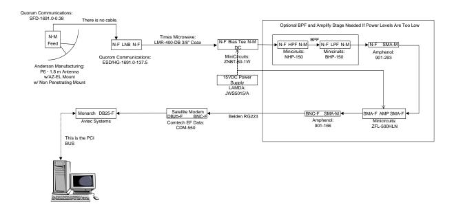
The above figure shows the basic connections for the LRIT User Terminal. The Domain 6 suite resides on the host computer and the LritReceiver uses the Monarch card to read the data from the satellite modern.
