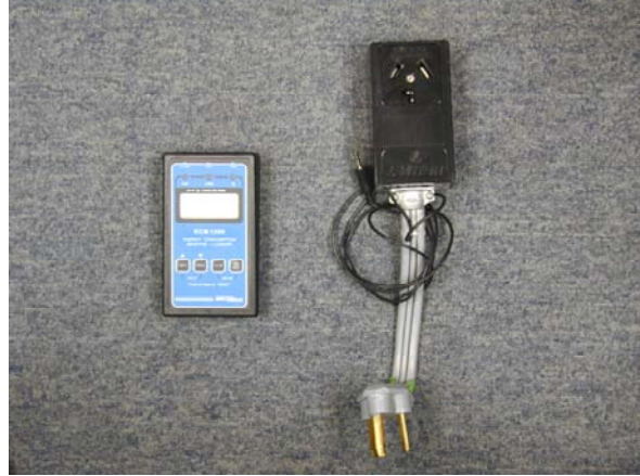
Figure 2.8 Dryer Energy Meter
