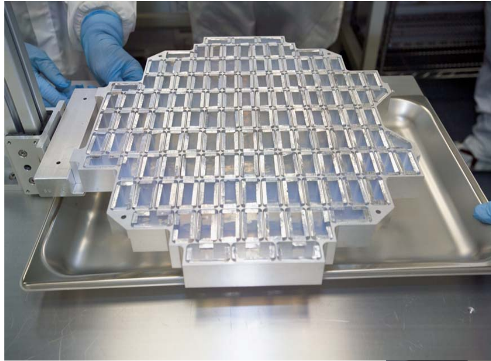
First close up view of the back side of the cometary collector
