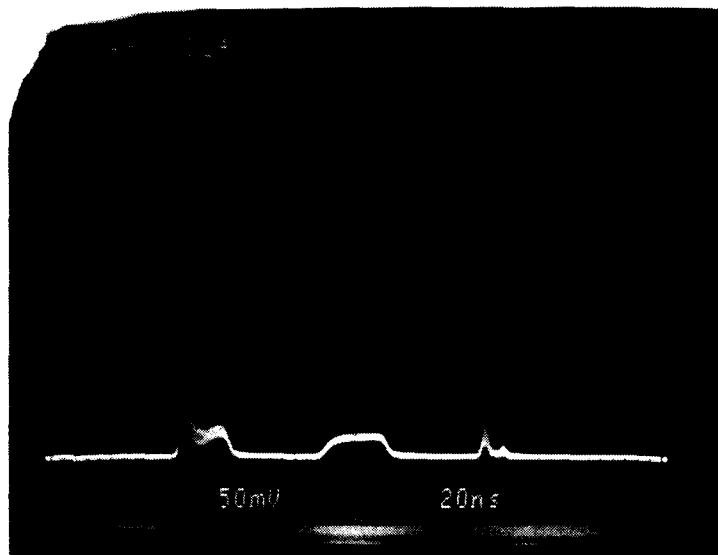
Figure 33: Receiver detector output with TU1 and TU2 "SET", TU3 "SET", TU4 "ON". TU3 aligned to remove circulator leakage and horn VSWR.
