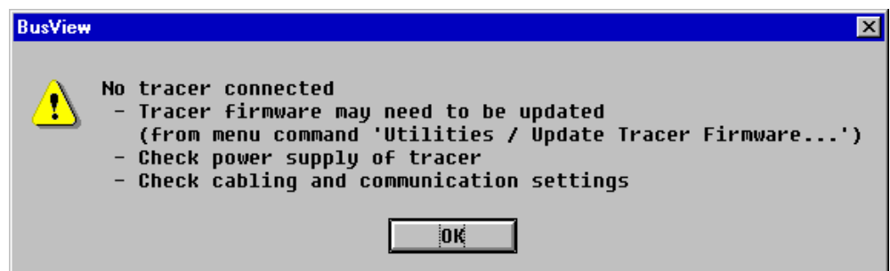
Figure 2.5 Warning message indicating that BusView was not able to connect to the VBT-325
