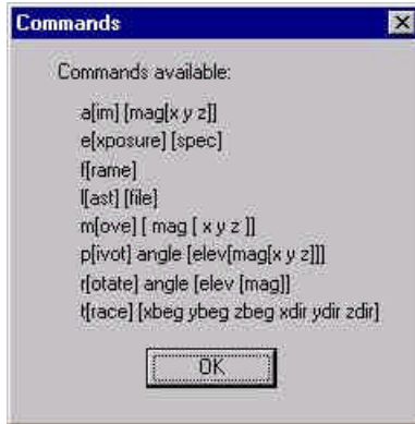
Figure 99. The available commands that can be used on the command bar in rview .
