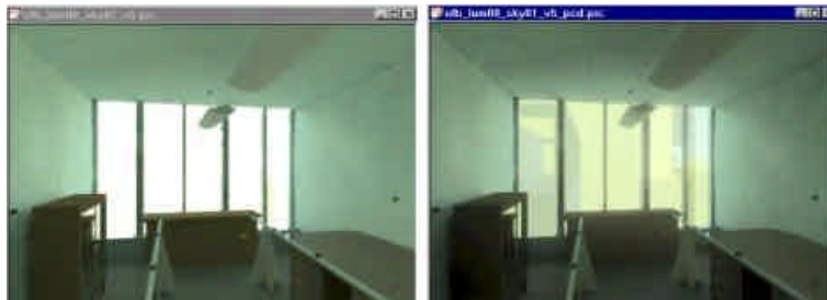
Figure 85. Image before (left) and after (right) running Human Sensitivity. Notice that Human Sensitivity image shows exterior details that are not visible in the other image.
