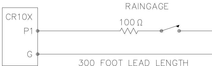
FIGURE 7.8-1. Wiring Diagram for Rain Gage with Long Leads
