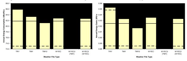
Figure 9 Comparison of Simulation Results in Seattle, WA, for Weather File Types and Actual Weather
