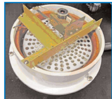
Figure 4.4.z New float and tiltmeter sensor
